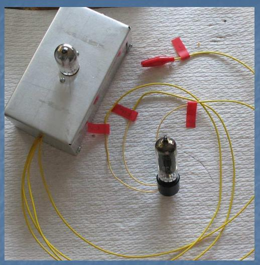
Pop out the 6CL6 first video amplifier and plug it into the socket saver.
