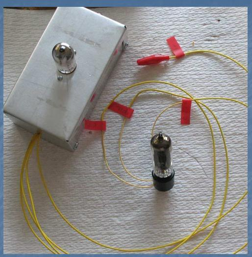
Only the B+ is obtained form another location. An insulated alligator clip connects the adapter to +275 volts at the above-chassis contrast pot.
