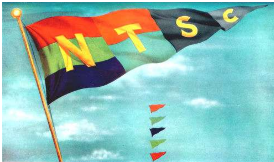
Plate VII. NTSC Flag illustrating color resolution in color television. Largest areas in full color as mixtures of red, green, and blue; smaller areas in cyan and orange; smallest details in black-and-white. (From Proceedings of the IRE, Second Color Television Issue, Jan. 1954. )
