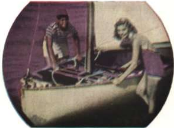
PLATE IV. Color television picture reproduced with Q signal but no I signal. (RCA.)
